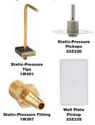
Static-pressure pickups mount to walls or ceilings and connect to pressure monitoring systems. 23Z320 is designed for cleanroom use. 23Z322 is for room mount with plastic enclosure that fits 2" x 4" electrical box. 23Z323 mounts on top of a standard ¾"-thick ceiling tile, with its filter facing down through a 5%" hole in the tile. 23Z324 is designed for roof or outside mounting, and is built to withstand harsh conditions.
