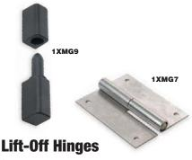
Surface-mount hinges allow quick door removal by lifting door from door-mounted hinge leaf. 304 stainless steel for use in corrosive environments. Black powder-coated, 300-lb, door capacity, 4 concealed mounting holes. Use #10 screws to mount; hardware not included.
